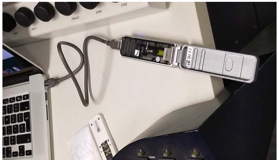
The Oxford Nanopore MinION system, a USB-sized cell that can be connected to a laptop, desktop computer or even a mobile phone.
