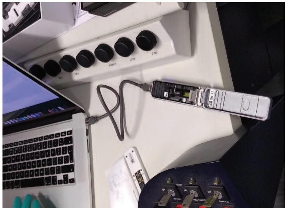
The Oxford Nanopore MinION system, a USB-sized cell that can be connected to a laptop, desktop computer or even a mobile phone.
